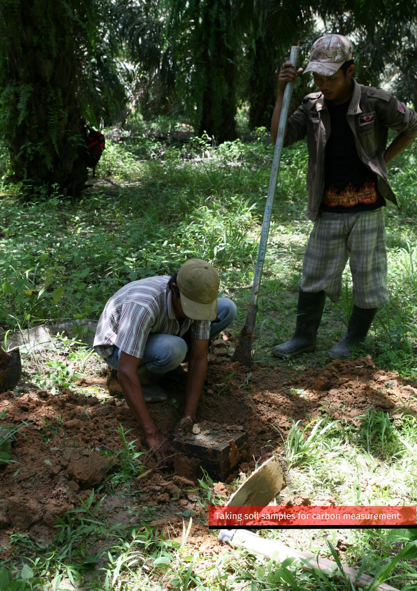
Taking soil samples for carbon measurement
