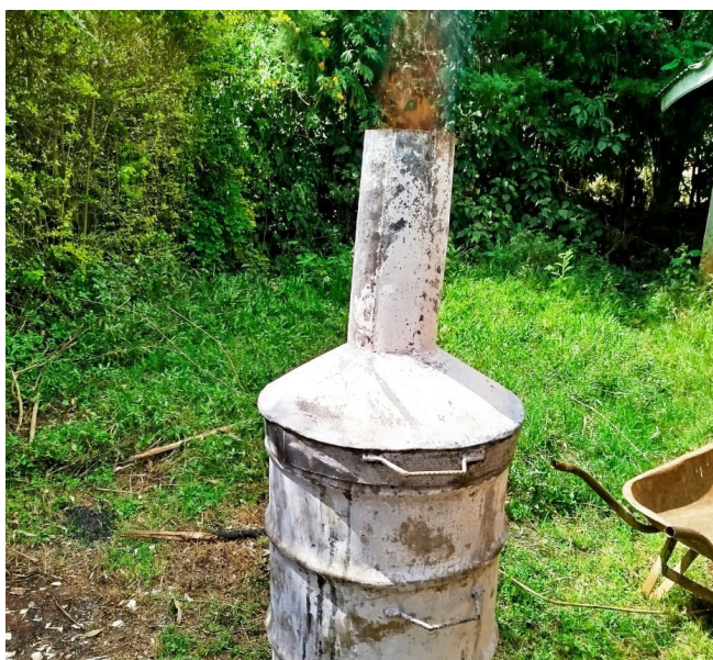
Figure 3. A kiln innovation that Mzee Mukoko uses for pyrolysis. Photo: © CIFOR-ICRAF/David Lelei
