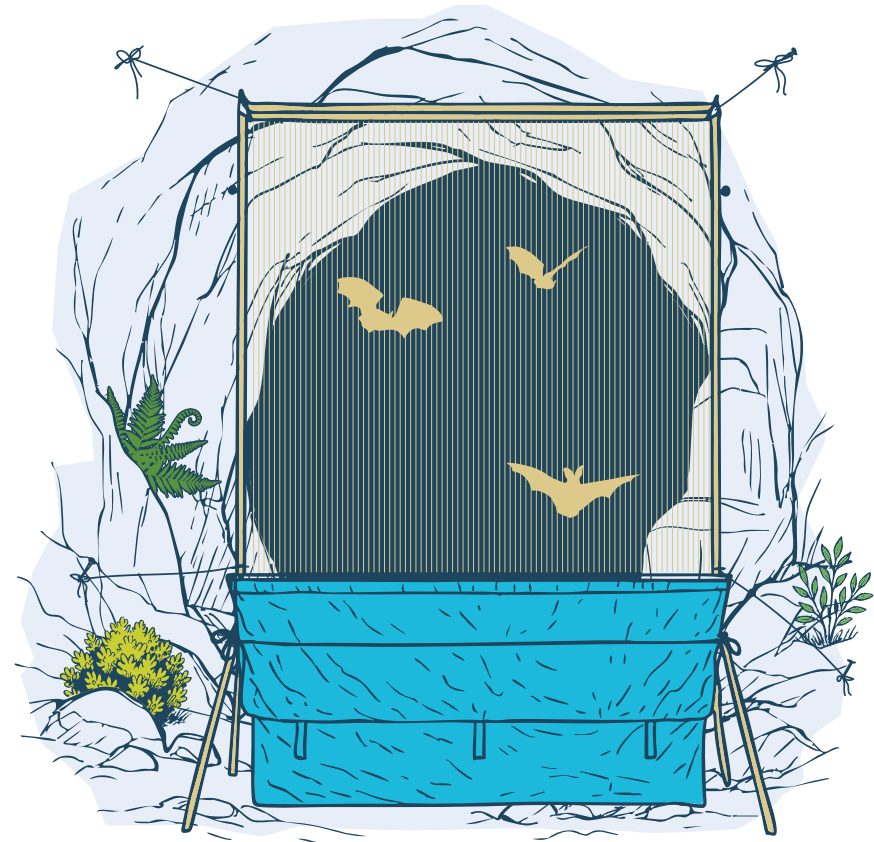
Figure 4. Sketch of harp trap setup for bats
