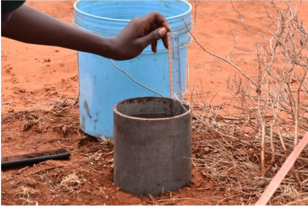
Figure 14: Infiltration measurement using a single ring infiltrometer.
