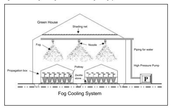
Figure 1. The design of the greenhouse with the fog cooling system
